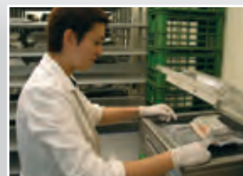
Archipress Vacuum packing machine in use for 'Squelch Drying' flood damaged materials.
