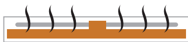
Aluminium layer subject to oxidation from ozone and reactive oxygen. Damaged disc will be unable to play
